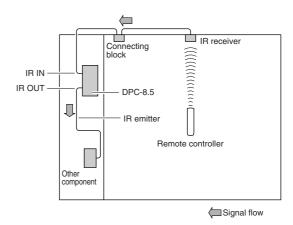
Connect the IR emitter to the DPC-8.5's IR OUT, and place the IR emitter in front of the other AV component's remote control sensor (usually located on its front panel), as shown below. See the instructions supplied with the IR emitter.
